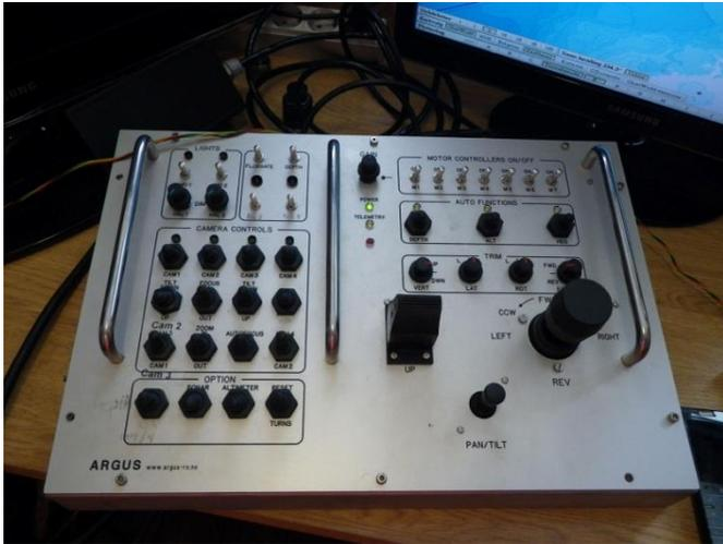
*Figure 4. Control panel of the Argus ROV*
