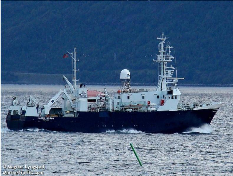
**Figure 6.** R/V “Hakon Mosby” equipped with Kongsberg EM3002D multibeam sonar used for bathymetric survey in the Norwegian Sea (courtesy of [www.marinetraffic.com](http://www.marinetraffic.com)).
