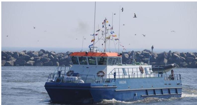
**Figure 7.** R/V “Varūna” equipped with SeaBeam 1185 multibeam sonar, used for bathymetric survey in the Baltic Sea (courtesy of [www.ve.lt](http://www.ve.lt)).
