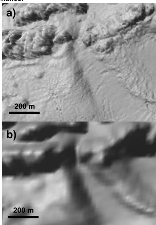
**Figure 10.** Raw multibeam bathymetry (a) and downsampled to models resolution (b). Note small imperfections present in raw data and not present in downsampled.
