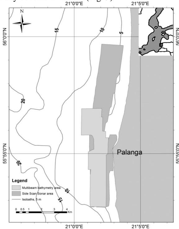
**Figure 9.** *Multibeam and Side Scan Sonar data collected in the Baltic Sea coastal area.*
