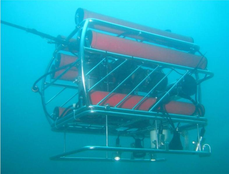
*Figure 2. The Mariscope ROV in use underwater.*
