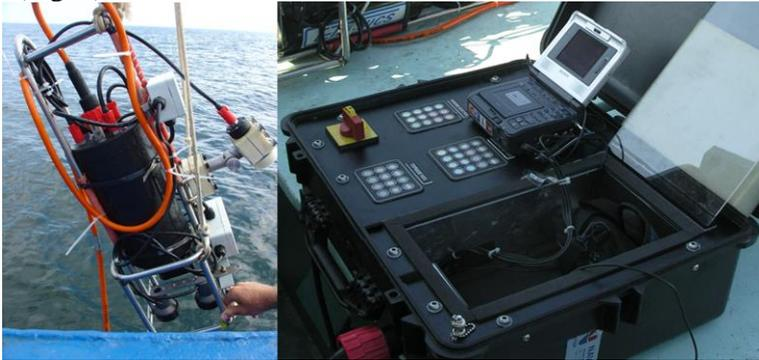
*Figure 1. Drop-down C-Technic remote underwater video system, underwater unit (on the left) and control box (on the right)*
