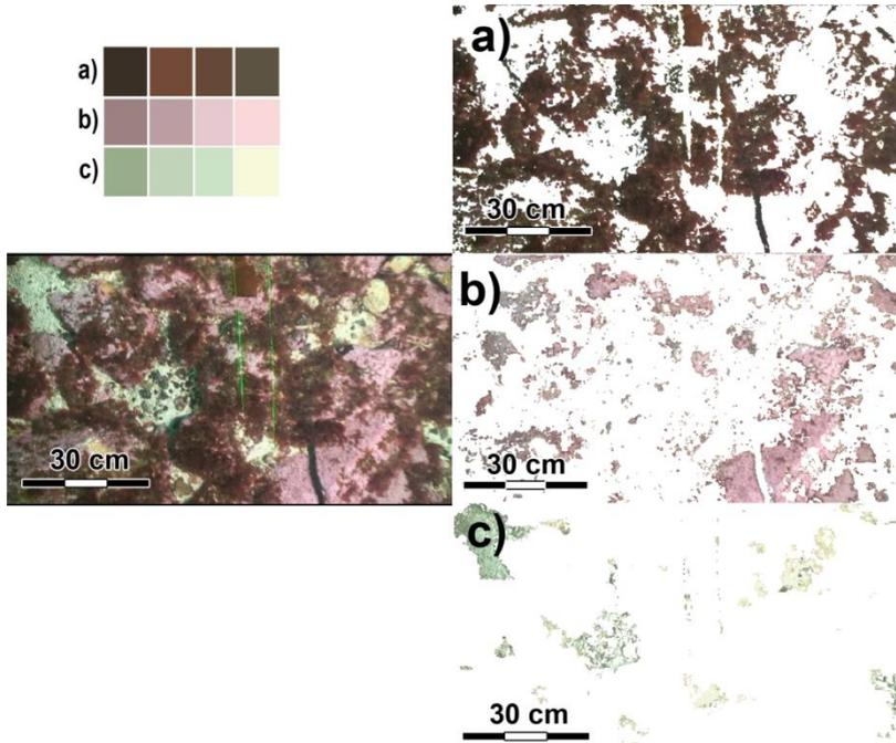
**Figure 7.** Benthic covers extracted by pixel colours. Raw frame to the middle left; a) extracted erect red algae layer; b) extracted *Lithothamnion* sp. encrusting algae layer; c) extracted sand layer. In top left, simulated colour palettes used to extract according benthic cover layers.
