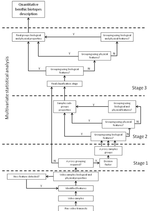
**Figure 13.** Procedure for quantitative benthic biotopes identification from underwater imagery used in this study. “Y” stays for “Yes”, “N” stays for “No”. Explanations in text.
