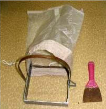
**Figure 4. The frame, mesh-bag and scraper were used to take biomass samples of *F. lumbricalis*.**
