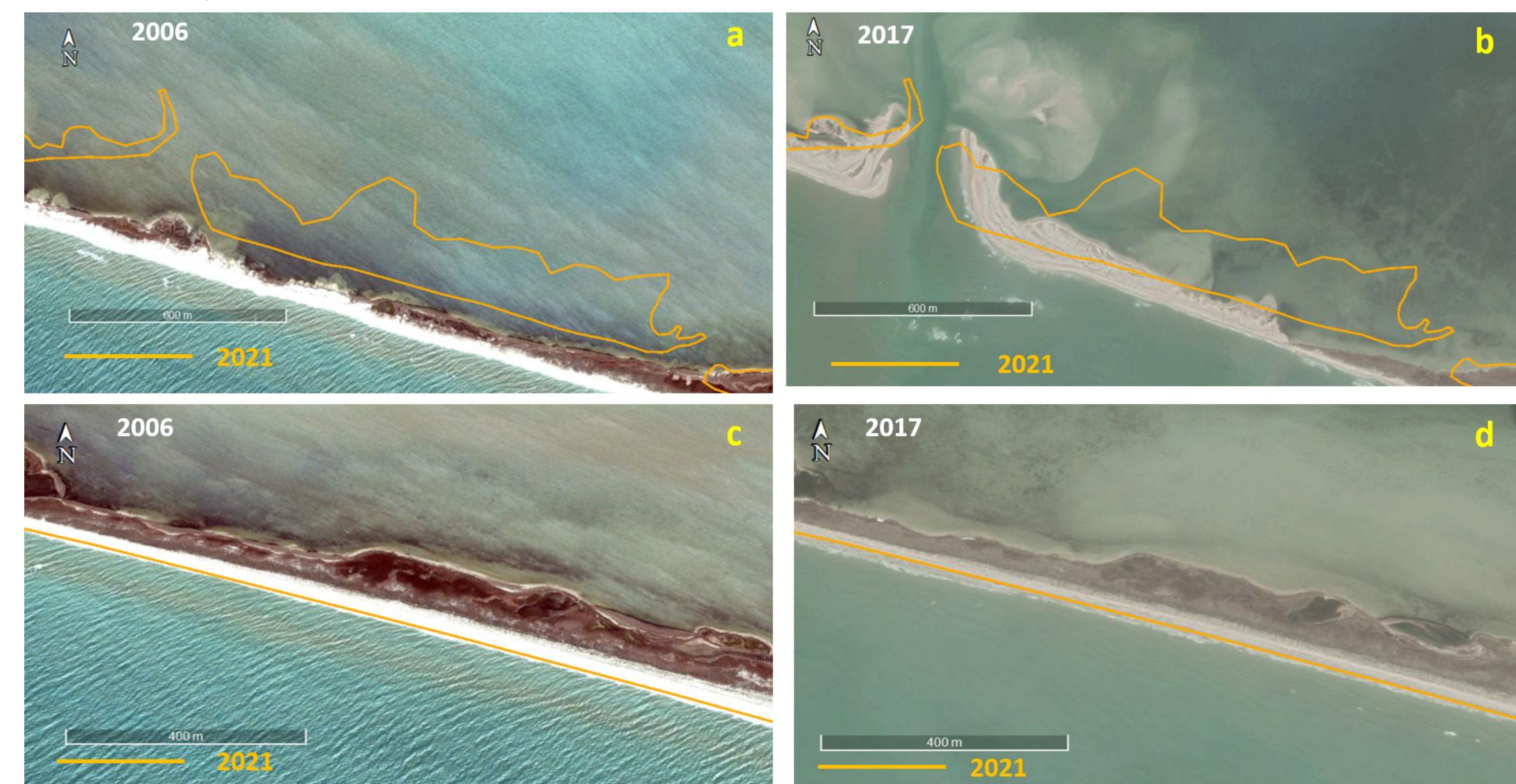
Features of the dynamic tendencies of the frontal coastline of the Tendra Spit: a - the state of the spit before the formation of the washout inlet; b - condition of the spit in the area of the inlet; c and d - the state of the spit outside the inlet formation zone.
