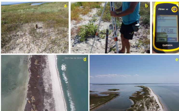
Fig. 1. Research methodology: a - stationary benchmark; b - geomorphological survey; c - GPS receiver; d - photo of the coastal barrier from an unmanned aerial vehicle; e - photo of the barrier from the quadcopter.
