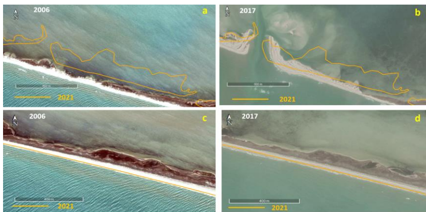
Fig. 2. Features of the dynamic tendencies of the frontal coastline of the Tendra Spit: a - the state of the spit before the formation of the washout inlet; b - condition of the spit in the area of the inlet; c and d - the state of the spit outside the inlet formation zone.
