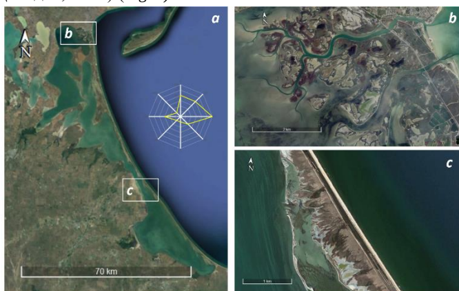
Fig. 2. Washout formations of the Arabat: a – appearance of the Arabat and the structure of the wind regime; b – modern washout formations the Tonkiy and the Promoina straits; c – area of the former scours of the Shokalinsky narrowing (developed by the author based on the Google Earth resource).
